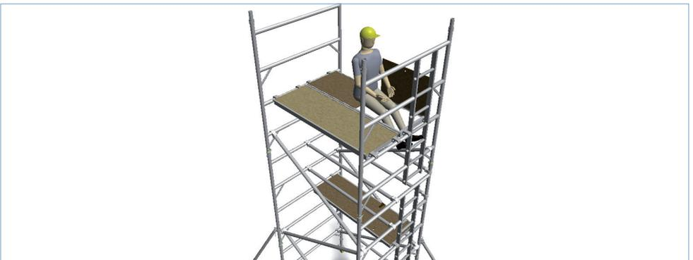
**1.36** Climb ladder and open trapdoor. Sit with feet through the platform with both feet on the ladder. Fit four guardrail braces on the 9th & 10th rungs directly above the sides of the platform.
