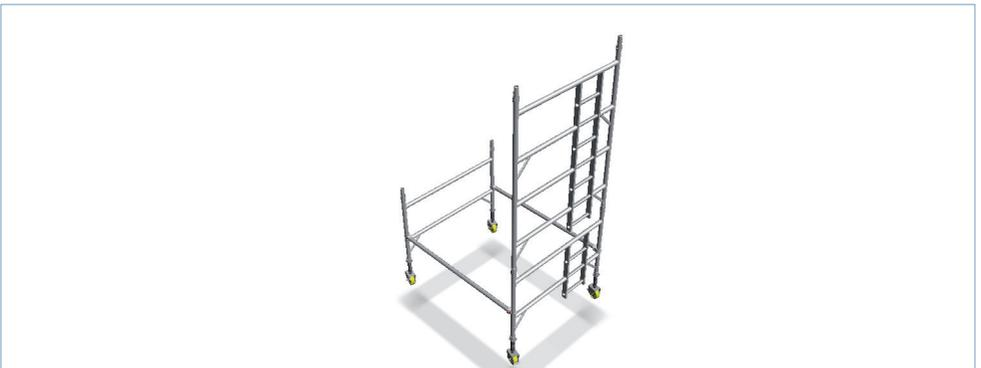
**1.9 Clip diagonal braces onto the lowest rungs.**
