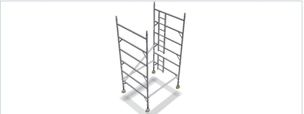
**1.11 Clip diagonal braces onto the lowest rungs.**
