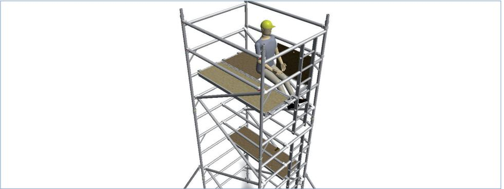
**1.43 Stand on platform and ensure that guardrails are securely in place at the opposite ends of the tower.**
