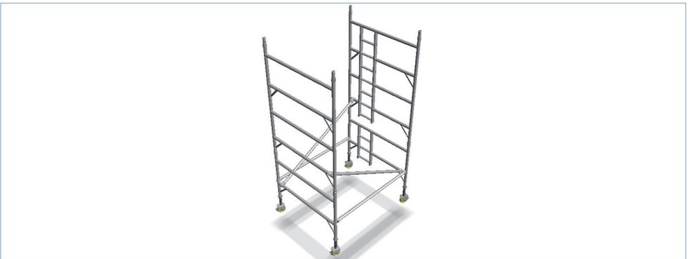
**1.12** When fitting the stabilisers, position each one in opposing directions. Adjust all four castors to ensure the tower is square and level. Use a spirit level.
