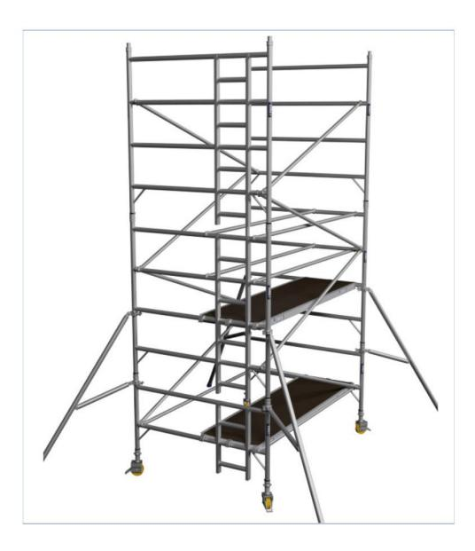
1.11 Remove the Temporary deck from the bottom rung and place it on the 8th rung with a trapdoor deck alongside it, with the hinges towards the outside of the tower, and the trapdoor next to the ladder.
