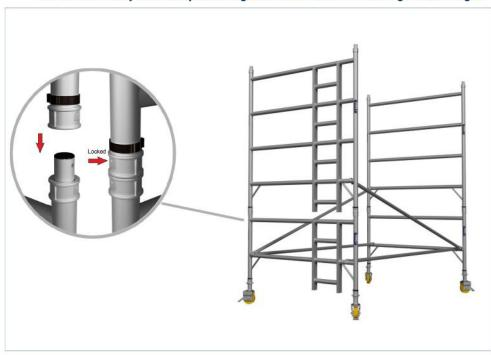
1.6 Make sure that the trigger is facing to outside of frame.
