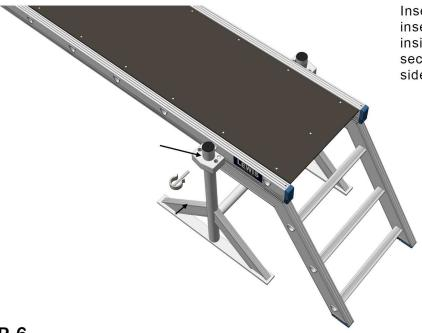
Insert the pins inside of the rung, now you've inserted the pins make sure they are safely inside of the rung and the staging board is secure so it cannot be shaken, ensure both sides are completed
